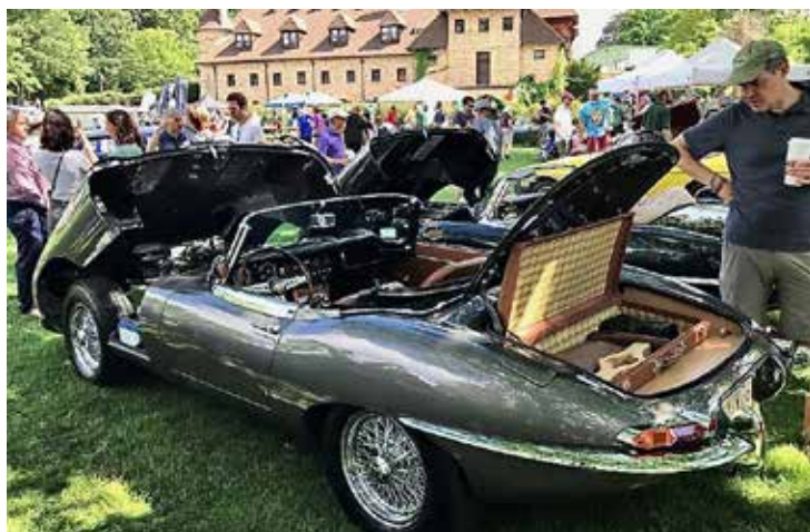
This spectacular E-Type took four years at a German restoration center to bring back to glory. It even had a custom-made tool box in the boot. The wooden form in the box is designed to surround the wire wheel spinner, so that it can be more easily loosened with a mallet.
